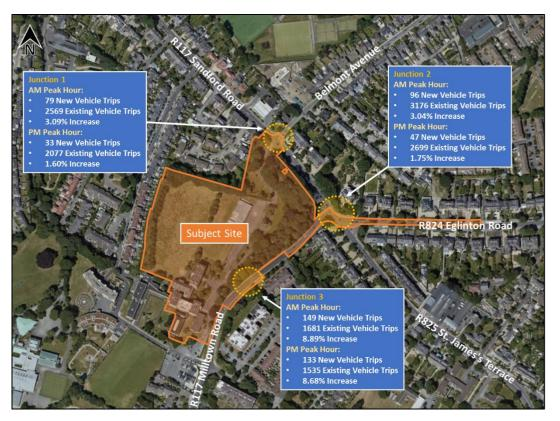
Figure 7.1: Increase in Vehicle Trips Generated Through Key Site Junctions
