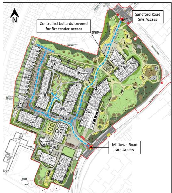
path analysis for the fire tender route has been shown on **DBFL Drawing 190226-DBFL-RD-SP-DR-C-1002.**
